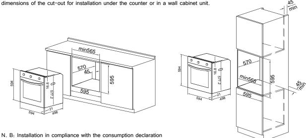
In order to ensure adequate ventilation, the back panel of the cabinet unit must be removed. Installing the oven so that it rests on two strips of wood is preferable. If the oven rests on a continuous ,flat surface ,there must be an aperture of at least  $45 \times 560$ mm.
